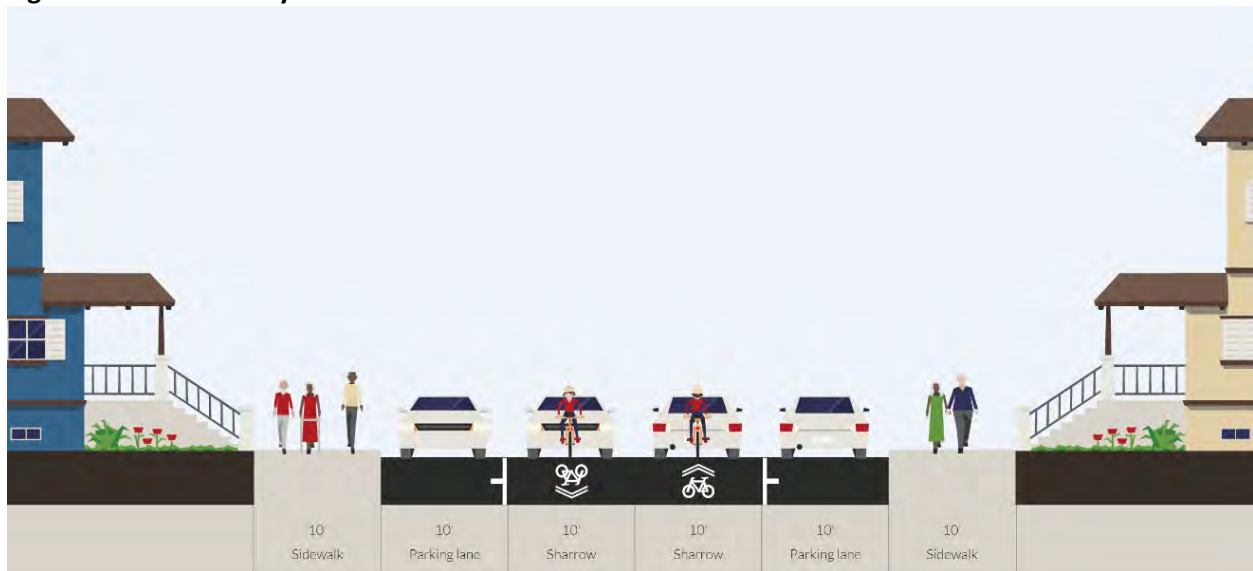
Figure 35. Sharrow Bicycle Route on Town Center Street
